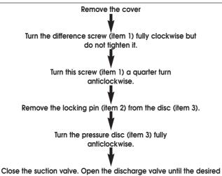
dry-running pressure is reached (read on pressure gauge).
